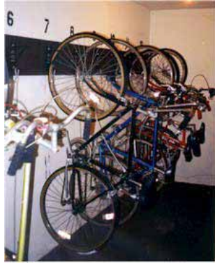
When vertically staggered, hanging racks can be spaced as close together as 17" on center.
